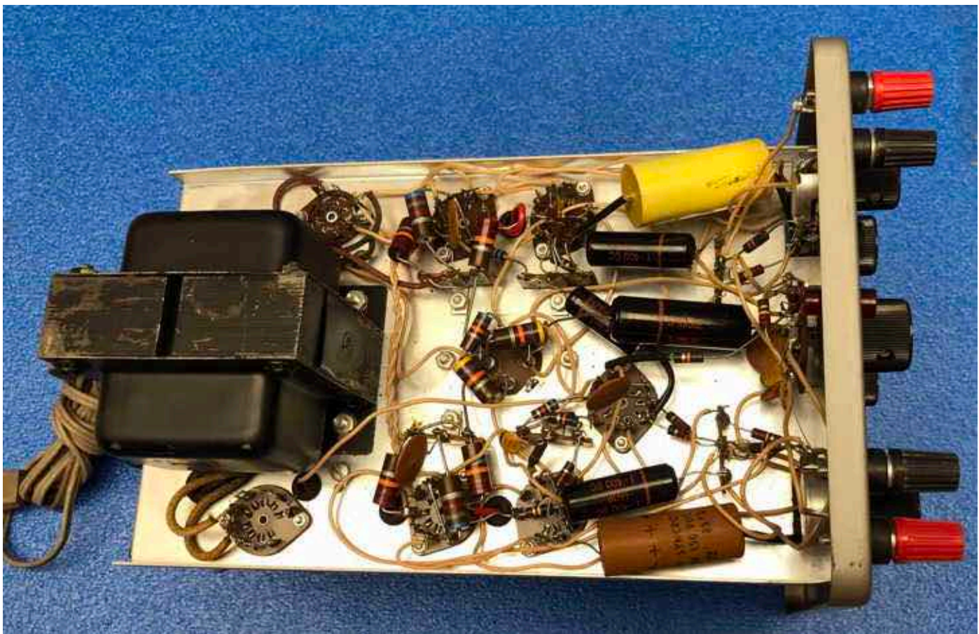
Figure 8: Heathkit IO-21 chassis bottom. photo. Note large power transformer towards rear. 1V2 HV rectifier socket is below the transformer, and 6X4 B+ rectifier is above. Large yellow and brown capacitors are the vertical and horizontal coupling capacitors respectively. Vertical amp is on top; horizontal is on bottom. B+ filter capacitor and sweep multivibrator are in the middle.
