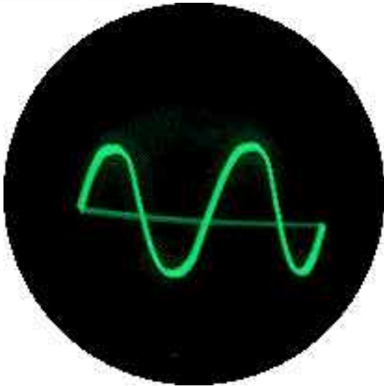
Figure 2: Scope trace showing the lack of retrace blanking. Note the almost horizontal retrace line connecting the trace start to the trace end.
